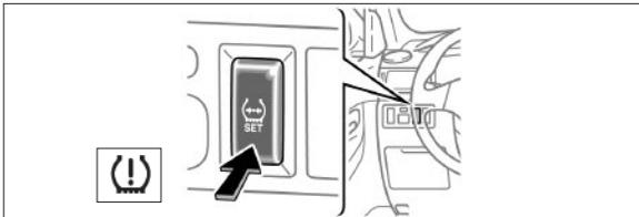
If tire pressure becomes critically low on any of the tires (excluding compact spare), indicator comes on. Pushing “SET” button should not turn off the light. Correctly adjusting tire inflation will turn off the light after a few minutes. After replacing tire or wheels, push and hold “SET” button until the indicator blinks 3 times.
