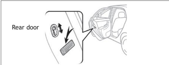
Moving the lever to “LOCK” will allow the door to be opened only from the outside.
