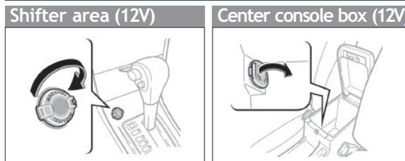
Designed for 12V car accessories. Key must be in the "ACC" or "ON" position to be used.
