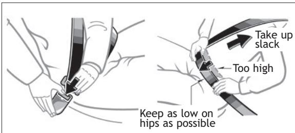
If belt is fully extended, then retracted even slightly, it cannot be re-extended beyond that point, unless fully retracted again. This feature is used to help hold child restraint systems securely.
