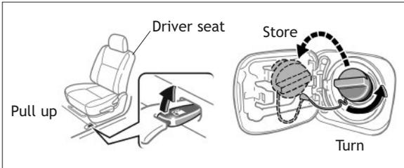
**NOTE:** Tighten until one click is heard. If the cap is not tightened enough, Check Engine “
