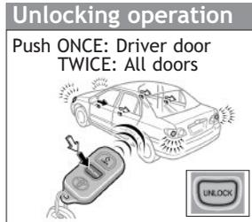
**NOTE:** After unlocking, if a door is not opened within thirty (30) seconds, all doors will relock for safety.
