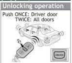
**NOTE:** After unlocking, if a door is not opened within thirty (30) seconds, all doors will relock for safety.
