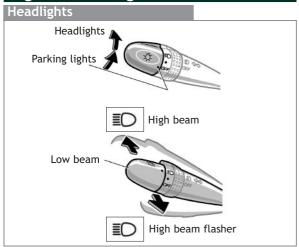
**Daytime Running Light system (DRL)** Automatically turns on the headlights at a reduced intensity.
